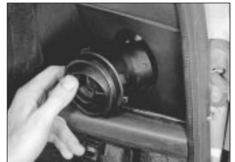
13.2 Turn the air vent anti-clockwise to remove
