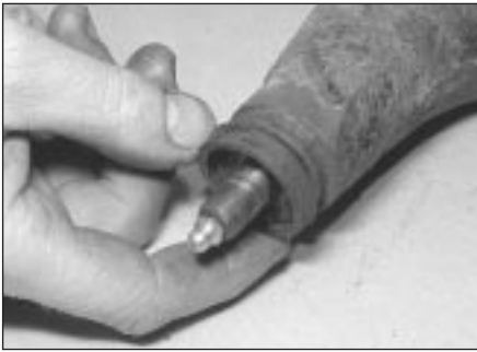
19.12a Lift off the radius arm bearing rubber seal . . .
