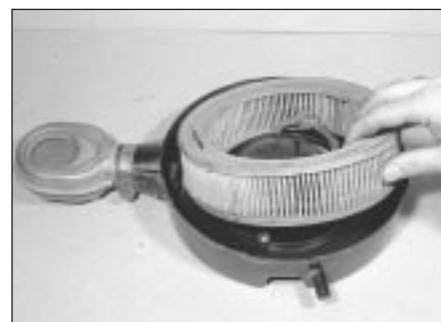
30.6b . . . and lift out the element
