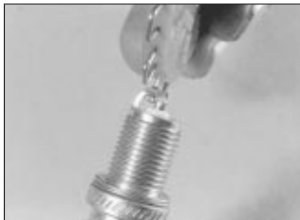
33.11 Adjusting a spark plug electrode gap
