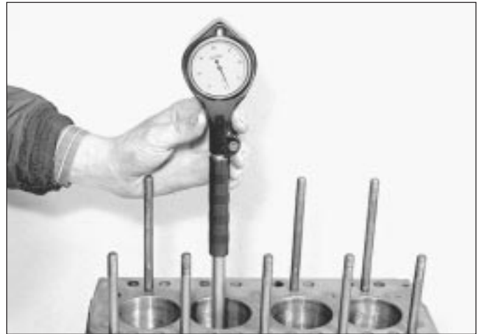
13.12 Using a bore gauge to check for cylinder bore wear
