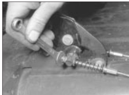
21.3 Remove the handbrake cable adjusting nuts
