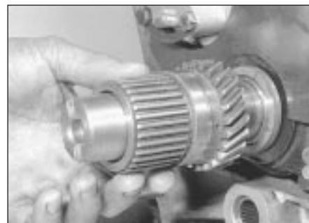
5.30 Slide on the primary gear ...
