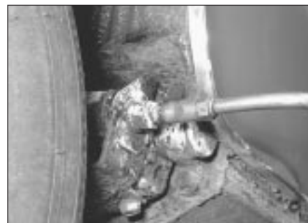
16.1c . . . and the rear radius arm pivot grease nipple
