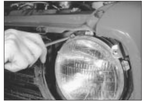
5.4a Unscrew the inner rim securing screws . . .
