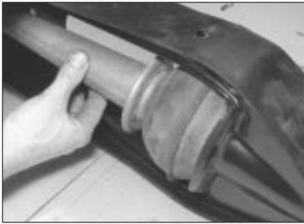
15.3 Remove the rear rubber cone spring strut . . .
