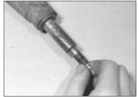
19.12c . . . then slide out the pivot shaft
