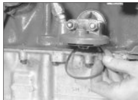
13.12 Fitting a new cartridge type oil filter sealing ring
