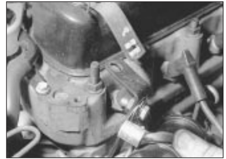
8.20 Remove the nut and release the ignition coil bracket
