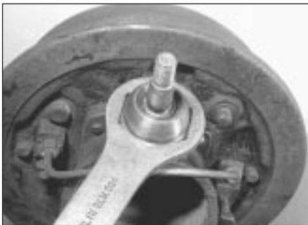
5.12c ... and fully tighten the nut
