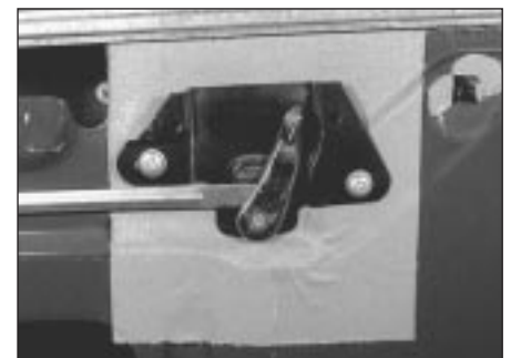
10.3 . . . the interior lock control retaining screws . . .
