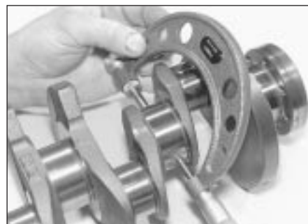
12.17 Use a micrometer to measure the crankshaft bearing journal diameters
