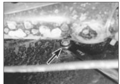
7.10 Removing the lower fan mounting nut (arrowed) - fuel injection models
