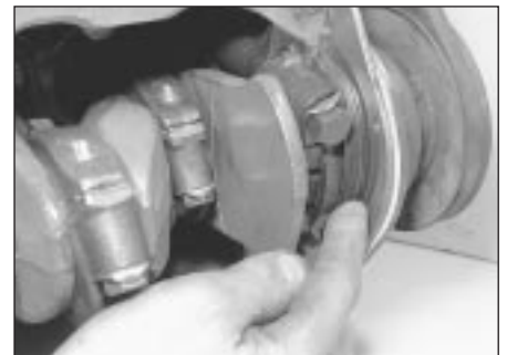
5.25 Fitting a new front oil seal . . .
