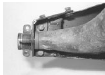
19.9 Rear radius arm outer bracket retaining bolts (subframe shown removed)
