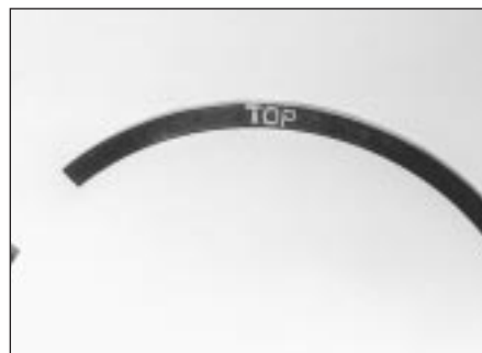
16.3 Piston ring identification markings
