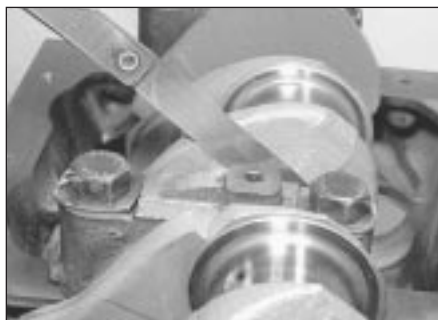
12.3 Checking crankshaft endfloat using feeler blades
