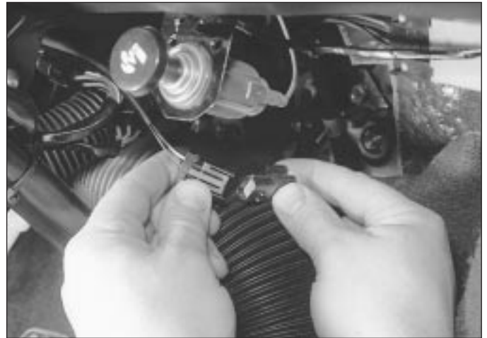
13.47 Disconnect the wiring connector . . .
