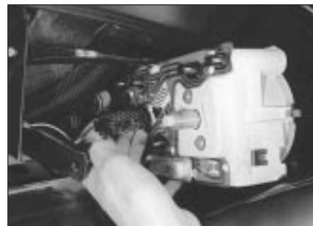
15.28b ... and the multiplug connector, then lift away the instrument panel
