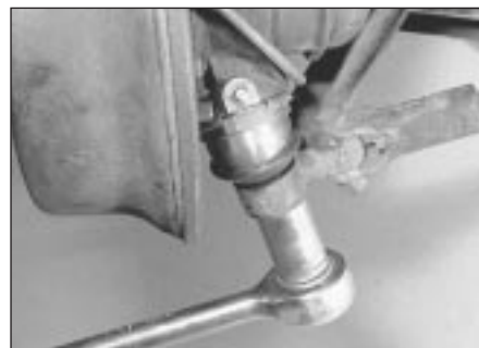
3.6 Remove the lower swivel hub balljoint retaining nut
