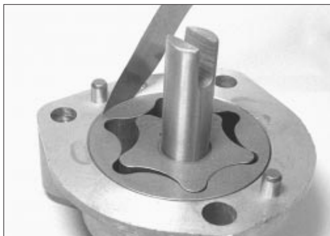
10.5b . . . and rotor-to-body clearance
