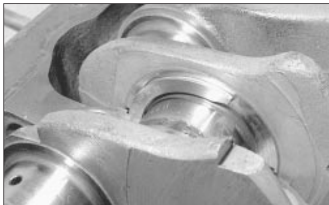
17.19 Refitting the crankshaft thrustwasher upper halves
