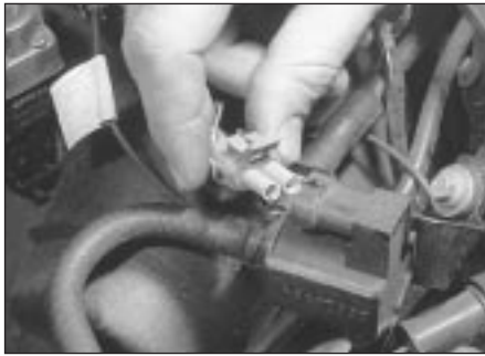
6.28 Disconnecting the purge valve wiring connector
