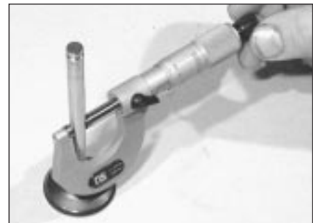
8.17 Measuring the valve stem diameter
