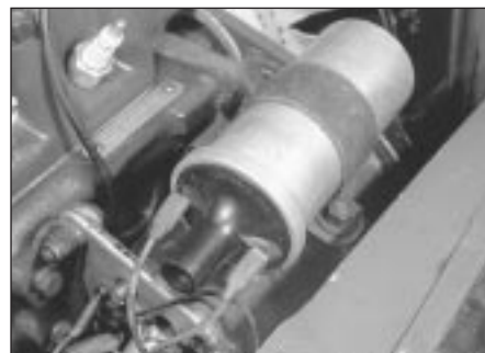
6.3 Disconnecting the coil leads
