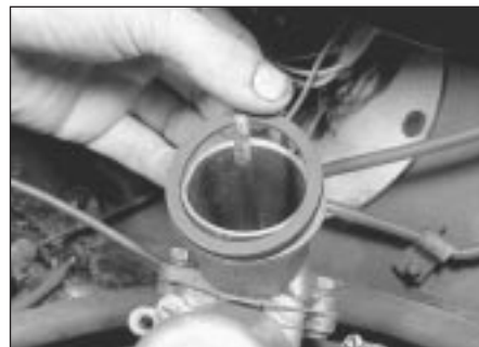
2.2b Recover the sealing ring
