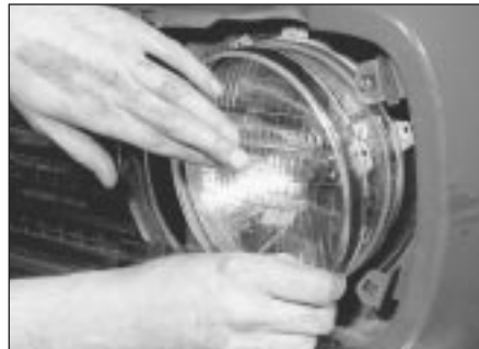
5.4b . . . and lift off the inner rim
