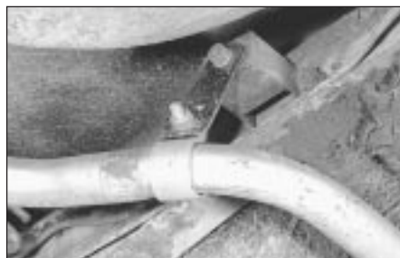
7.2a Exhaust front mounting block . . .
