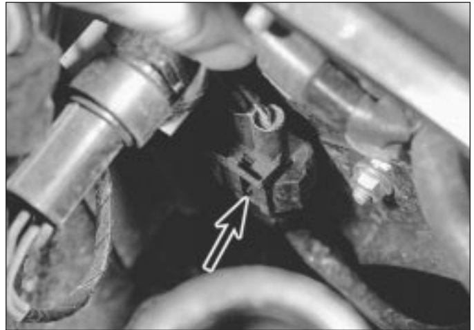
7.9 Auxiliary fan motor wiring connector (arrowed) - fuel injection models
