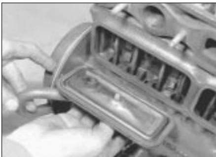
9.1 Removing the tappet side covers
