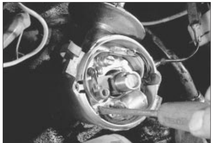
5.7 Adjusting the contact breaker points
