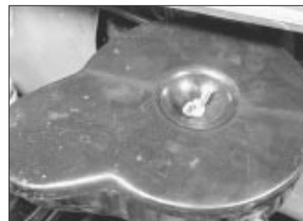
2.1a Remove the single wing nut on early models . .
