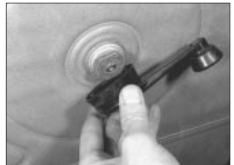
6.2b . . . and the window regulator handle
